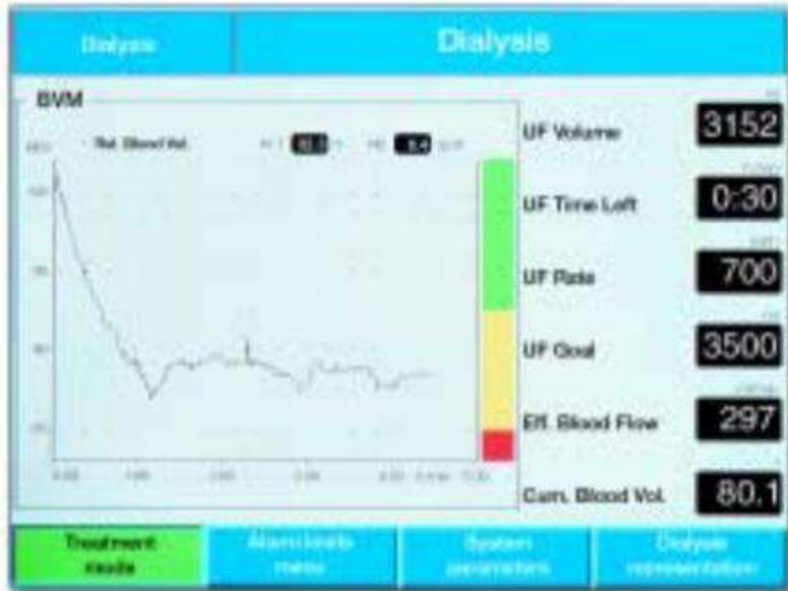
Fig. 11: RBV during a BV controlled treatment in the display of the 4008 dialysis machine
